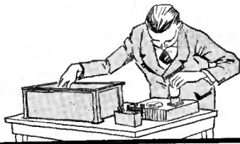
In series-filament circuits much time may be saved by testing the continuity of each tube filament separately with a C battery.
