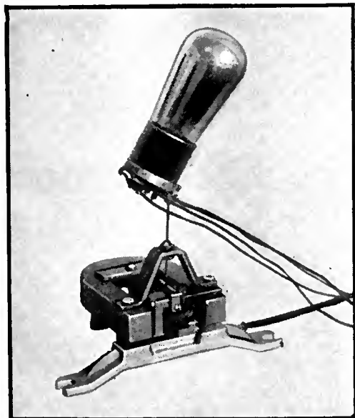
A vibrator unit employed in tests to determine the conditions under which vacuum tubes are microphonic.
